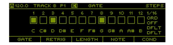
This page allows editing the currently selected sequence on the currently selected track. Depending on the track mode of the selected track, this page shows a different graphical representation of the sequence. If track mode is set to *MIDI/CV*, the page is not available and selecting it will jump to the Track page.
