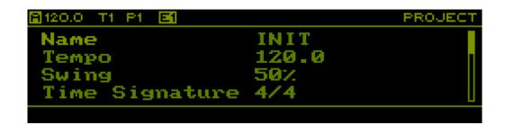
This page allows to change project wide parameters as well loading and saving projects from/to the SD card.
