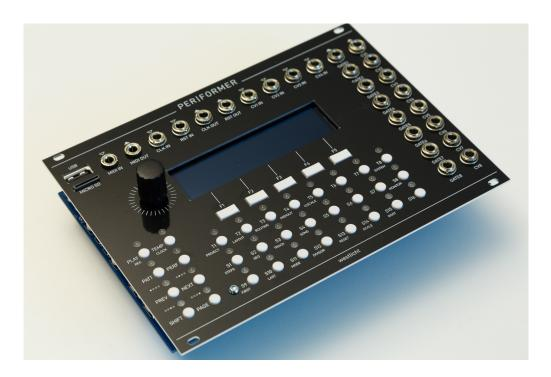
**PER|FORMER** is an open source and open hardware eurorack sequencer module. It packs a lot of functionality into a small form factor and was designed both as a versatile sequencer in the studio as well as for live performance. To fully take advantage of all the features available in this module, it is highly recommended to study this document carefully.
